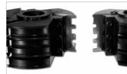
**Charles G. G. Schmidt & Co.** has introduced a new insert style surfacing head for the flooring industry. These aluminum heads are made with four or six rows of standard four-sided inserts to do the surfacing, and two dovetail slots to accept adjustable cutters for adding the relief cuts on the bottom of the flooring. When used with the company's flip-flop design insert-style side heads, once the machine
